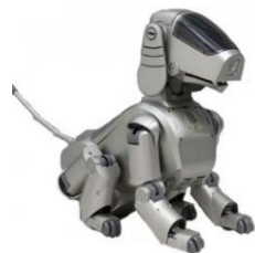
Fig. 1. When Sony’s AIBO was first released in 1999, it included a 64-bit processor, 16MB of RAM, and an array of sensors for creating the robot’s personality.
